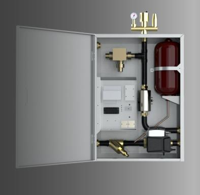
Power World's Hydrobox makes heat pump installation and maintenance easier. Hydrobox integrates water pumps, small expansion tank, valves, safety components, electric heater, and other components. When installing the heat pump system, the installer can connect the heat pump directly to the Hydrobox, which is very simple and convenient, even if you do not have a lot of experience, you can follow the instructions to complete the installation
