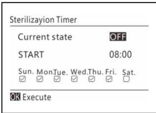
If the current status is 'off', clicking the 'OK' button will manually activate the sterilization function (the set timed sterilization is still effective).
