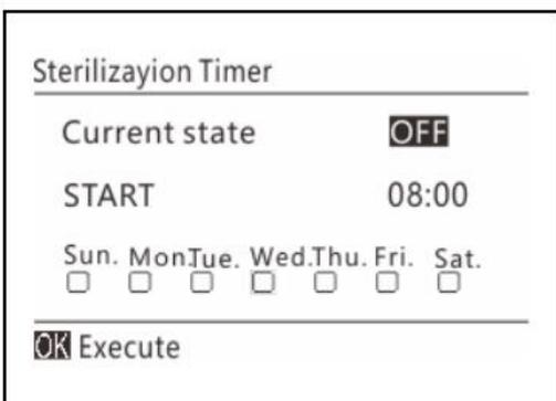
First, use the "Up", "Down", "Left", and "Right" keys to move the cursor and select the starting time point where timed sterilization needs to be enabled. Click "SET" to set it.
